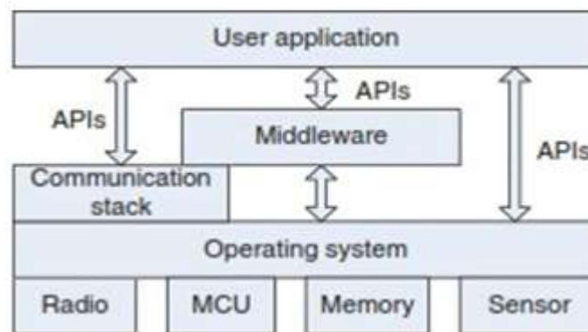
Figure 1 Generic architecture of a BAN Node [3].
